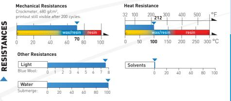
Evaluation of observed performances of the ribbon with optimised printer settings and receptors (ARMOR procedure).
